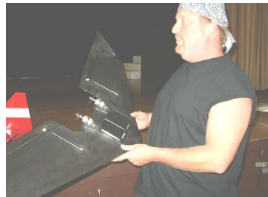
Chris has a prototype twin speed 400 flying wing that has been clocked at 72 mph.
